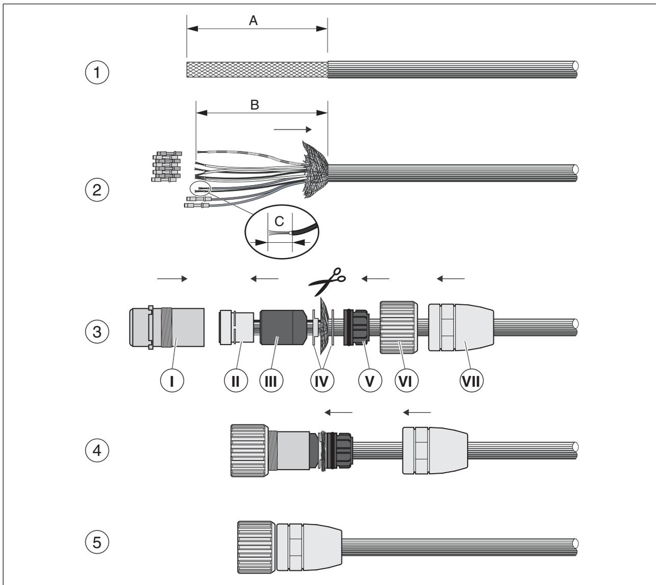
Figure 4.7 Assembling motor cables with M23 encoder connector
