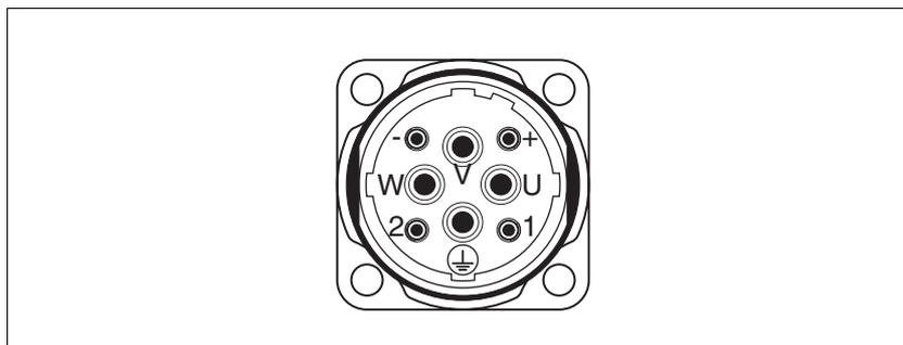
Figure 4.5 Pin assignment motor connection M40
