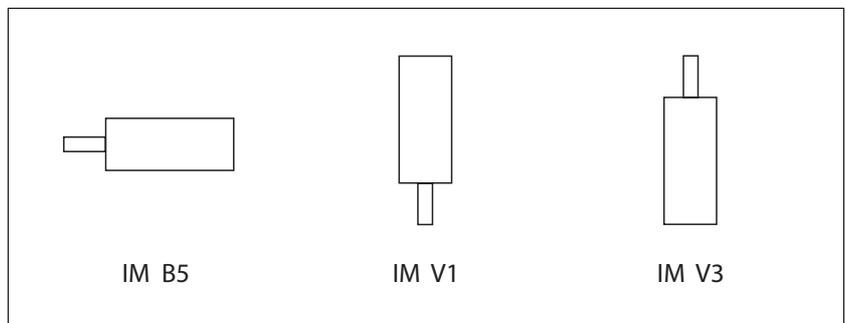
*Mounting* When the motor is mounted to the mounting flange, it must be accurately aligned axially and radially and evenly contact the surface. All mounting screws must be tightened with the specified torque. There must be no tension. See chapter 3 "Technical Data" for data, dimensions and degrees of protection (IP).
