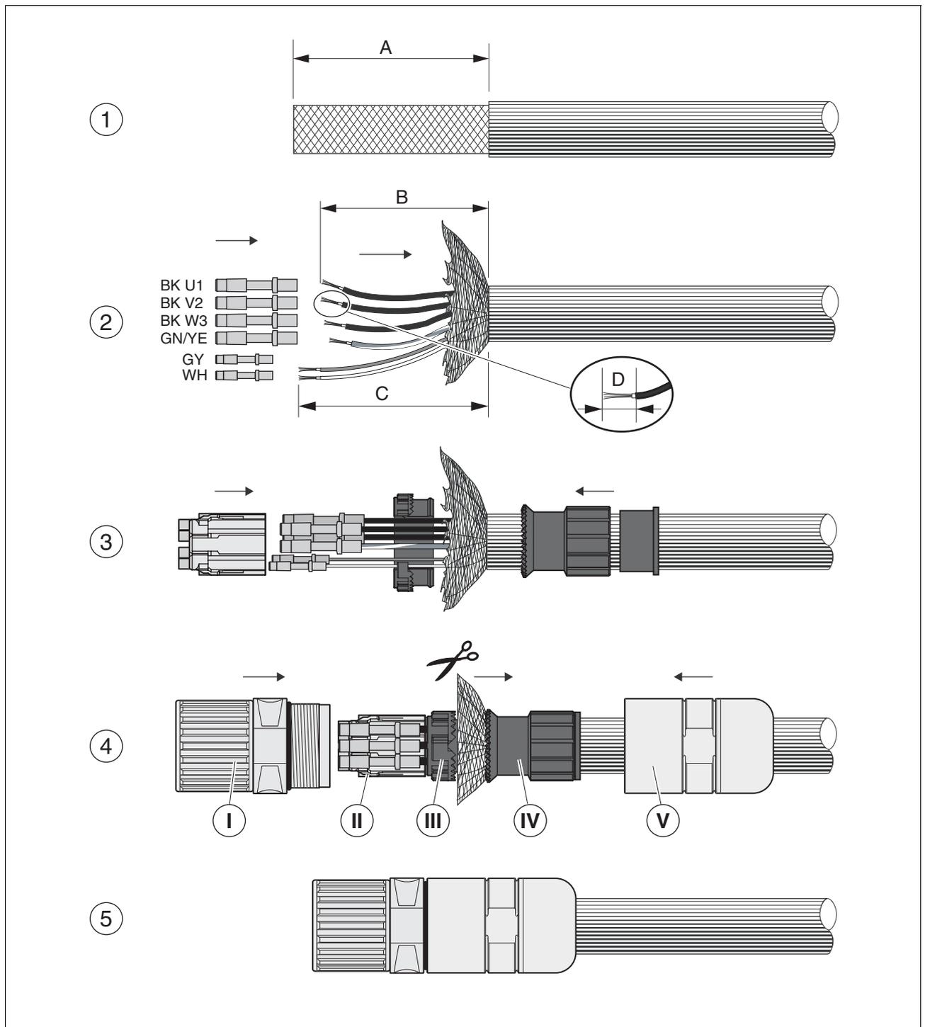
Figure 4.8 Assembling motor cables with M23 motor connector
