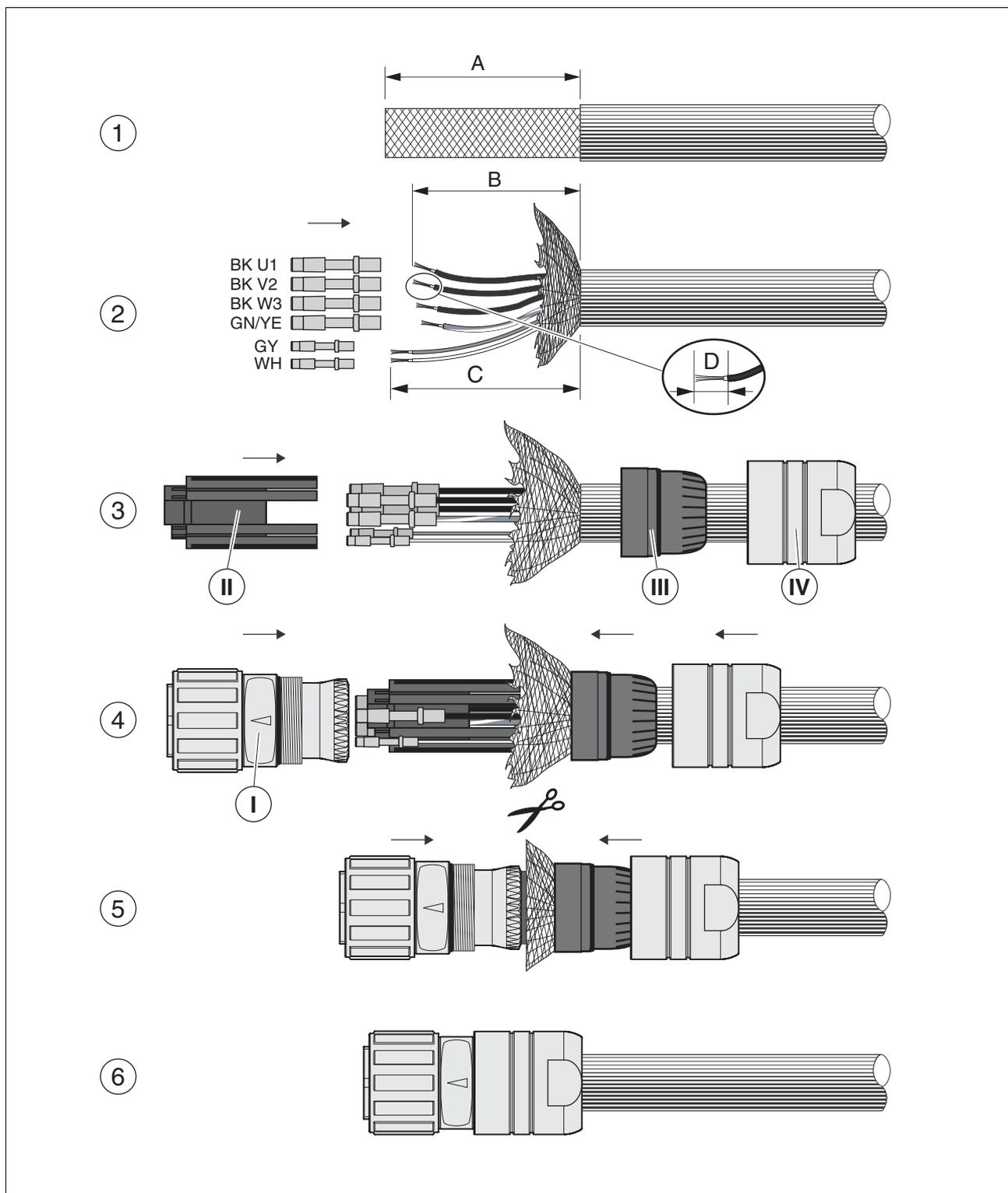
Figure 4.9 Assembling motor cables with M40 motor connector
