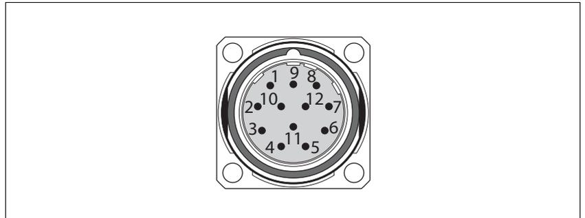
Figure 4.6 Pin assignment encoder connector
