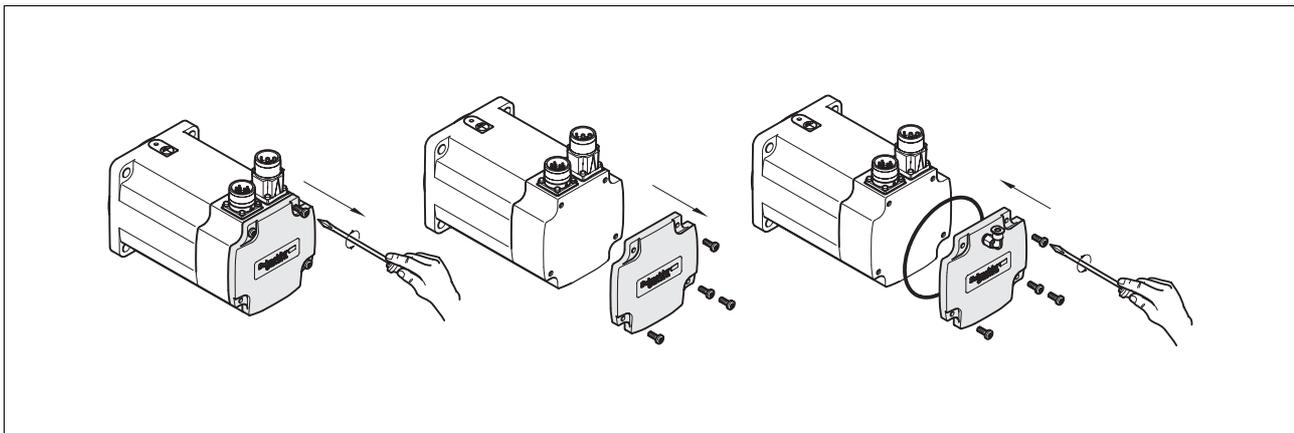
Figure 4.2 Installation IP67 Kit
