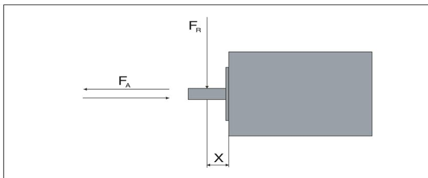
Figure 3.5 Shaft load
