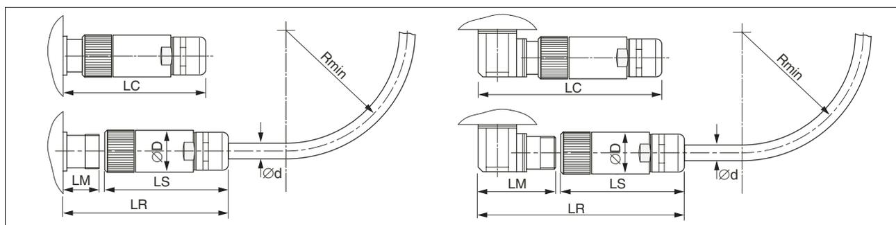
Figure 4.1 Connector installation space
