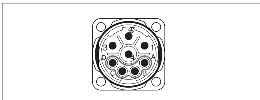
Figure 4.4 Pin assignment motor connection M23
