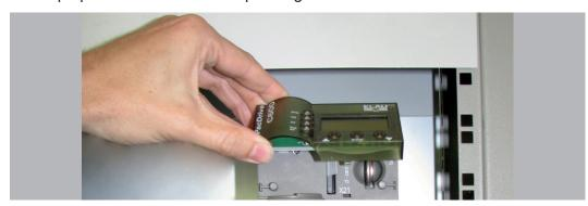
▶ Undo the two fastening screws on the front of the controller (1).
