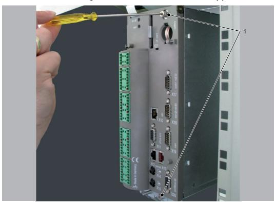
▶ Then remove the electronic module from housing.
