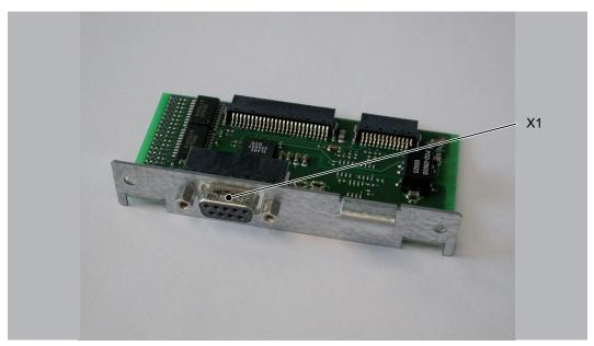
Following installation, the controller automatically detects the optional module. You then configure it using the control configuration in EPAS-4.
