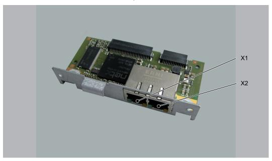
Figure 10-1: OM-NE module with slot assignment
